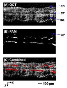
Fig. 3. *x-z* cross-sectional images of a mouse ear obtained by (A) OCT and (B) PAM. (C) Overlay of (A) and (B). ED, epidermis; CT, cartilage; SG, sebaceous gland; CP, capillary.
