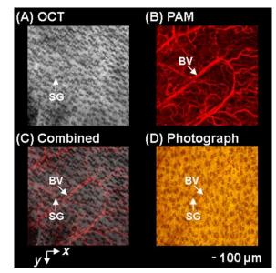
Fig. 2. *x-y* projection images of a nude mouse ear obtained by (A) OCT and (B) PAM. (C) Overlay of (A) and (B). (D) Photograph taken through an optical microscope. SG: sebaceous gland; BV: blood vessel.
