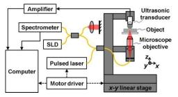
Fig. 1. Schematic of the combined photoacoustic and optical-coherence microscope. SLD: superluminescent diode. Solid lines represent single-mode optical fibers. Arrowhead solid lines show data flow. Arrowhead dashed lines show the flow of system control signals.
